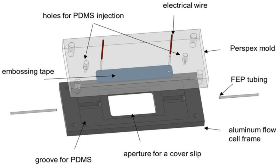
**Fig. 1** Components of the flow cell chamber. A custom-built Perspex mold is mounted onto a custom-built aluminum flow cell frame that holds a  $24 \times 40$  mm cover slip. Subsequently, PDMS is injected into the chamber between the mold and the groove of the metal frame
