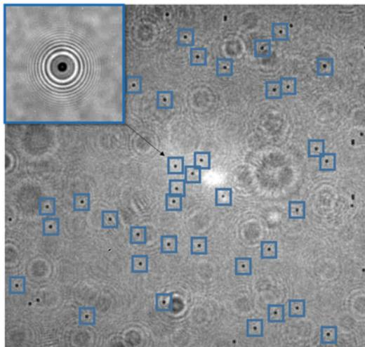
**Fig. 7** Selection of beads before tracking. Distribution of tethered magnetic beads on the imaged region of a flow cell. Small regions of interest (ROIs) were selected to track the diffraction rings of individual magnetic beads. Inset: a zoom of one of the selected ROIs
