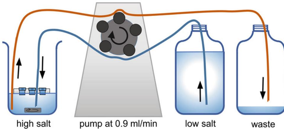
**Fig. 3** Schematic representation of the dialysis system controlled by a peristaltic pump. Samples are dialyzed against a high salt buffer. Subsequently, a low salt buffer is pumped into the beaker with dialyzed samples, while an equal volume is flown out into a waste bottle to ensure a constant volume and a gradual decrease of salt concentration in the dialysis tubes
